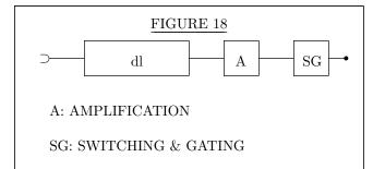
dl is to be used as a memory its output must be fed back—directly or indirectly—into its input. In an aggregate of many dl organs—which M is going to be—we have a choice to feed each dl back into itself, or to have longer cycles of dl 's: Figure 19 (a) and (b), respectively.
