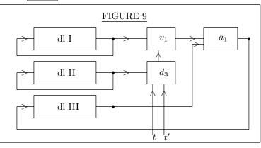
clearly have to contain dl-like elements (cf. {}). (b) The k (delay lengths) of the dl I – dl III. These too have certain functions of synchronization: Each time when the adder functions (that is in each interval it-ft) the multiplicand and the partial product sum (that is the outputs of dl I and of dl III) must be brought together in such a manner that the former is advanced by t (moved by one position to the right) relatively to the latter, in comparison with their preceding encounter.
