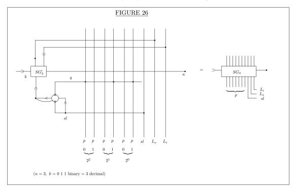
The input and output  $\supset$ — and —• at the left end of DLA correspond to the  $\supset$ — and —• of Figures 18, 23 (*a* and *c* of Figure 20), they can be connected up in various ways, as shown by the alternatives of Figure 19.—but at any rate DLA can only function if the circuits are closed in some way between these  $\supset$ — and —•.
