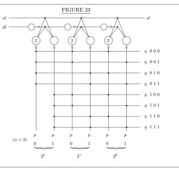
two vertical *p*-lines issuing from this group: 0 or l if the digit was 1 or 0. i.e. a *p*-line will carry no stimulus if and only if it represents a digit equal to the k digit in the upper  $\bigcirc$  of the E-element trio from which it issues. Now the connections of the horizontal q-lines with the vertical *p*-lines make it clear, that a -line will carry no impulse if and only the digital symbol associated with it agrees with k in all its digits–i.e. if it is the *q*-line No. k.
