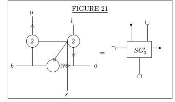
When SG' is on, a stimulus needs one period  $\tau$  to get from b to o, i.e. to  $L_o$  (cf. 13.3 and the end of this Section 13.4), and one to get from  $L_i$ , i.e. from i (cf. Figure 20) to a—that is, it takes  $3\tau$  from b to a. It is desirable that the timing should be the same when SG' is off, i.e. when the stimulus goes via  $\bigcirc$  from b to a—hence a triple delay is needed on  $\bigcirc$ .
