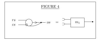
It should be noted that this  $\underline{m_1}$  corresponds to the actual vacuum tube trigger circuits mentioned at the beginning of 5.1. It is worth mentioning that  $\underline{m_1}$  contains one E-element, while the simplest trigger circuits contain one or two vacuum tubes (cf. loc. cit.), in agreement with the estimates of 6.5.
