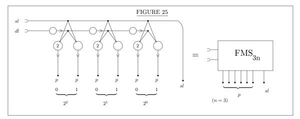
We redraw the central part of the function matrix switch accordingly: Figure 25 in place of Figure 24. The remaining parts of Figures 23 and 24, i.e. each q-line in its entirety, as described above, must be added to the corresponding SG. Actually we considered the sketch of SG in Figure
